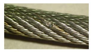
**Weld** - a rescue hoist cable can get so hot that it is annealed. Causes: static discharge, lightning.
