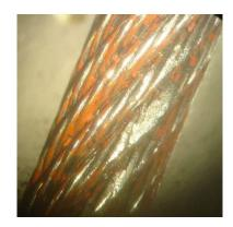
**Abrasion** – Abrasion is defined as wear of individual wires resulting in flattened areas on the wire. Abrasive wear can be caused by interference with other components, dragging the cable over abrasive surfaces, or as a result of other cable damage. Cables that have abrasive damage must be replaced and, if applicable, the cause of the abrasion must be investigated and repaired.
