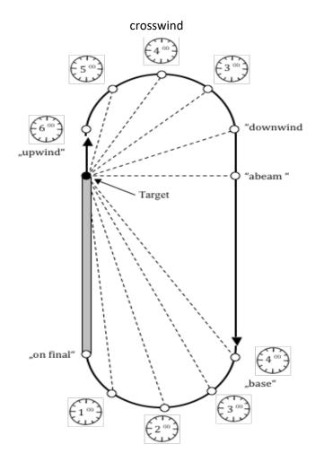
When approaching the operation site, a standard approach pattern is chosen. During this pattern, the helicopter is flying at a safe speed and at a safe altitude; all necessary briefings, preparation of the cabin and of the Rescuer take place during the pattern.
