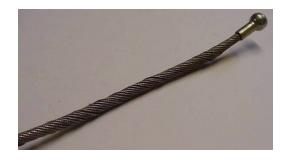
**Cable Milking** is a common end of life phenomena and is due to the action of the hoist tension rollers on the outer strands over a long period of time. When this appears after a long life the cable may be starting to fatigue, it should be replaced.
